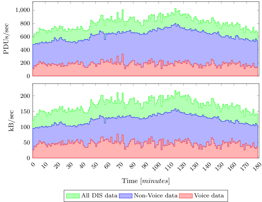
Figure 4: Packets per second and bandwidth utilisation for the duration of the exercises.
